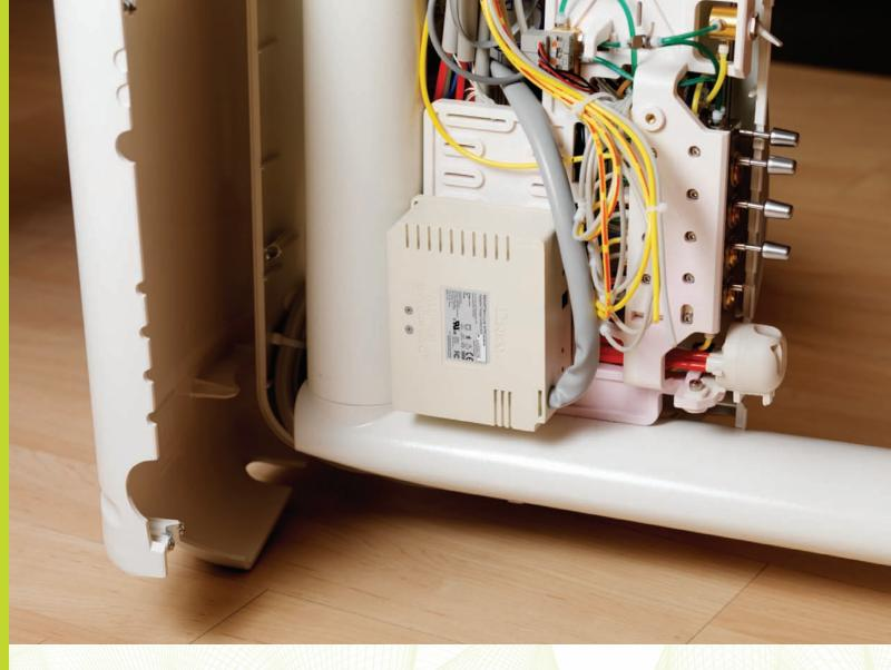
A-dec<sup>®</sup> 541 Connecting the Controller Main Air
